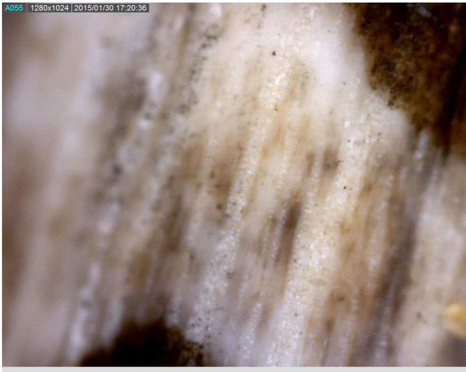
Figure 1035. The single zigzag bead (figure 1034) under Dinolite 200x magnification, showing remnants of the original tree that had not fully silicified
